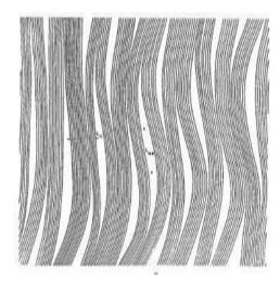
4. A crossplied FRP laminate, showing nonuniform fiber packing and microcracking (from B. Harris, Engineering Composite Materials, The Institute of Metals, London, 1986).[153]
