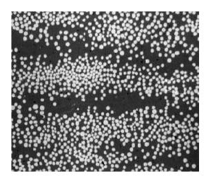
6. Photo micro graph of transverse ply cracking in a 0/90 GRP laminates.[152]
